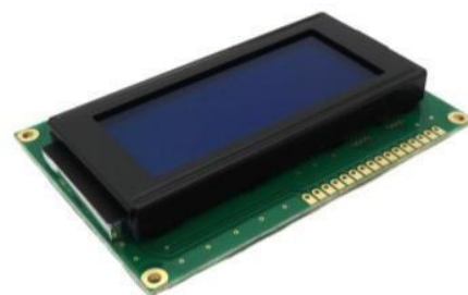
Gambar 2.7 LCD 20x4 I2C
