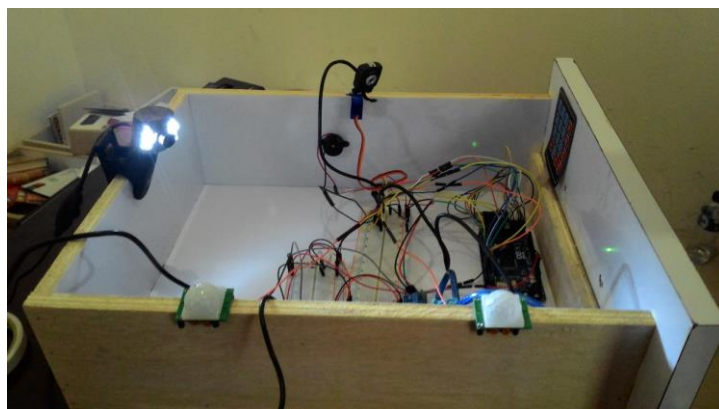
Figure 4.6 PIR position when sensor testing process
