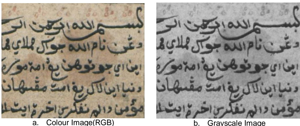
Figure 2. Changes of RGB image to grayscale
